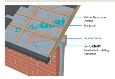
Starting at the bottom edge of the roof and working horizontally across the rafters, staple BreatherQuilt to the first rafter using minimum 14mm staples, pull taught and proceed across the roof.
